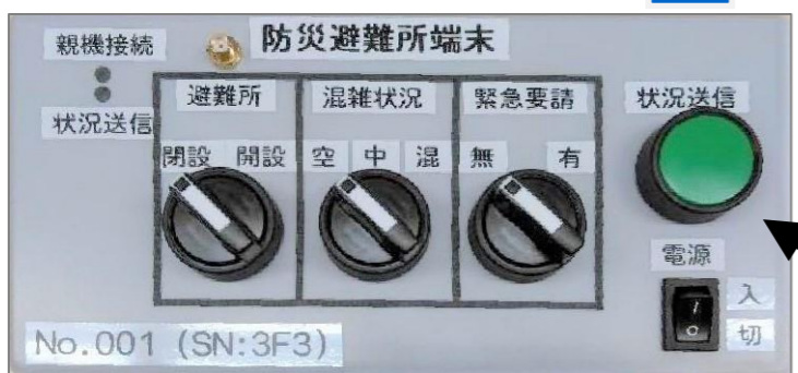
Shelter device, Shelter Monitoring equipped with LoRaWAN wireless
